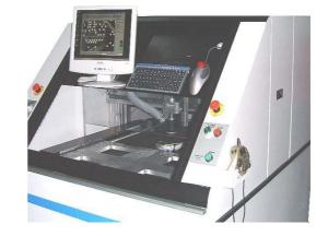
A separate vacuum hose allows the operator to use it as a vacuum cleaner during maintenance. All slides and leadscrews are protected against the abrasive dust by covers and bellows
